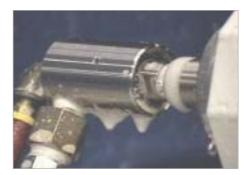
Installing the **ModulCLEAN** System couldn't be easier. Simply replace an idler roller with a 4, 6, or 10 inch diameter **ModulCLEAN** unit, and connect the water supply. A detergent/sanitizer supply can also be connected, if desired.
