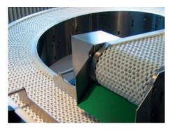
**Space saving** Small collapse factor of 1.6 that allows extremely tight turns and requires 30 percent less space than common belts with a collapse factor of 2.2.
